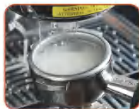
6. Remove the handle and press the pumping key to rinse the handle
