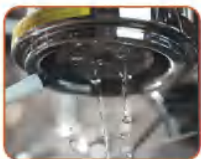
1. Use cleaning to brush off the coffee residue on the water network
